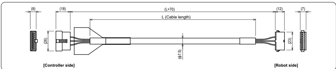
Signal cable (1500mm to 2600mm) Note. Common to MR types and MF types
