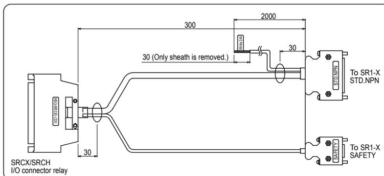
Note. It is necessary to input the 24V-power supply from the outside.
