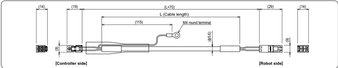
Motor wire (1500mm to 2600mm) Note. Not usable on MR type
