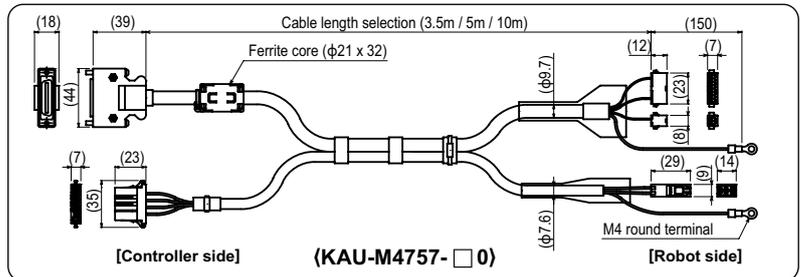
2-axes multi-robot cable
