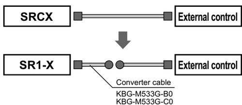
Converter cable allows connecting to the SRCX connector when system using the SRCX was changed to the SR1-X.
