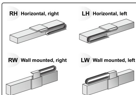
Note. Be sure to install in the direction as specified (in cable carrier take-out direction drawing and various specification drawings) individually. Installation in any other way will cause a failure. For requirement of installation in any way other than the above standard installation, please consult YAMAHA as special arrangement will be available.
