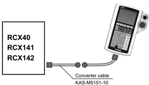
Converter cable for operating the RCX40, RCX141, RCX142 by RPB.
