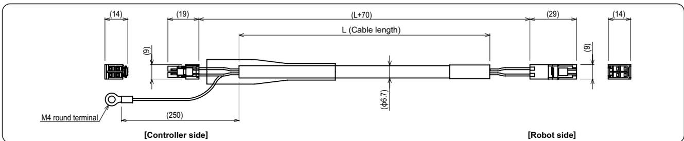
Signal cable (350mm to 1450mm) Note. Common to MR types and MF types
