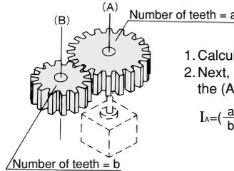
1. Calculate the moment of inertia  $I_b$  around the (B) axis.
