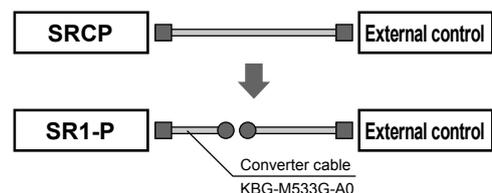
Converter cable allows connecting to the SRCP connector when system using the SRCP was changed to the SR1-P.
