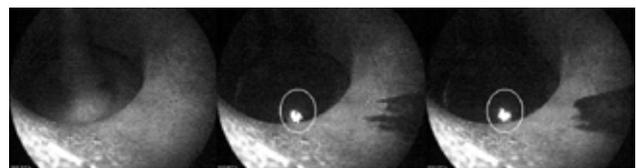
Figure 26 Wall film at intake valves under wide open throttle at every 2 cycle in System 3 at IVC. Circle: Flush light is visible in these images because of large wall film.
