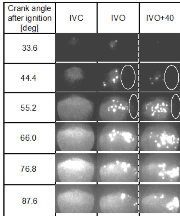
Figure 15 Flame propagation with different injection timing in System 2. Flame propagation is suppressed in the circles.
