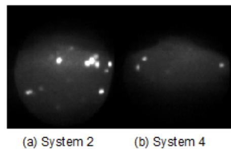
Figure 18 Images of flame at 32.4 deg aTDC under wide open throttle with injection timing of IVO+40.
