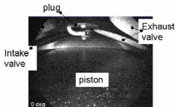
Figure 3 Actual field of view of combustion chamber.
