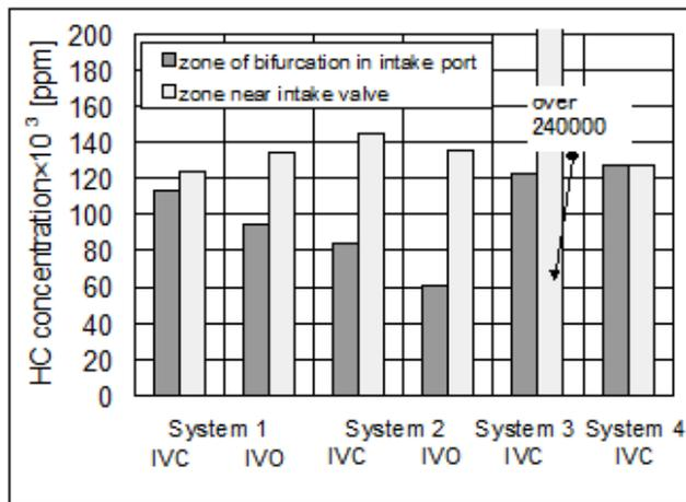
Figure 28 Hydrocarbon concentration, IMEP; 400 kPa.
