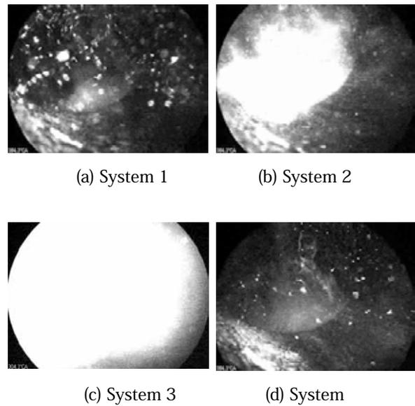
Figure 24 Spray images of view inside intake port at timing just before intake valve open with injection timing of IVC.
