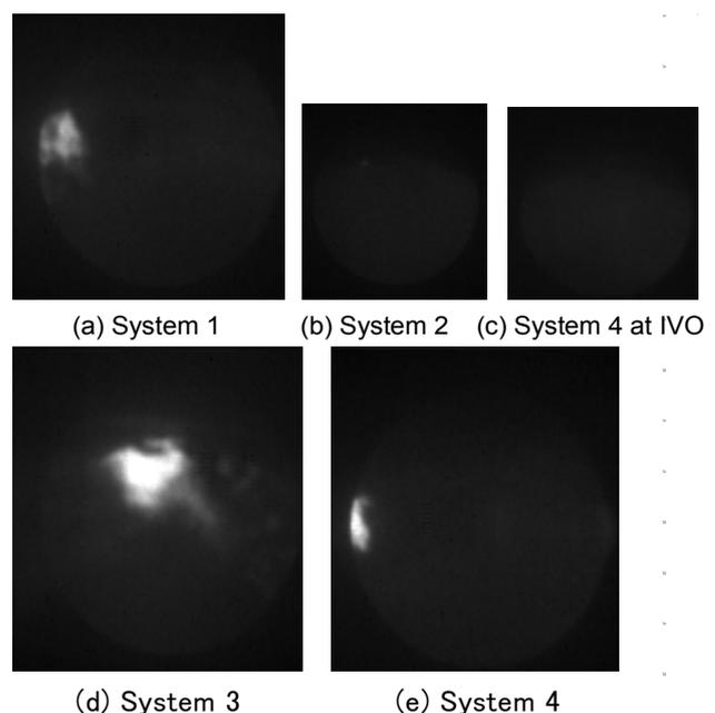
Figure 19 Flame images at 100.8 deg aTDC under wide open throttle with injection timing of IVC except (c).
