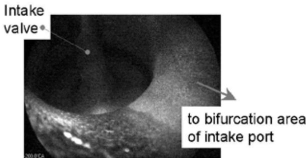
Figure 5 Actual field of view for intake port.
