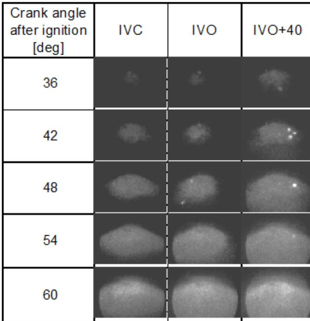
Figure 14 Flame propagation with different injection timings in System 4.
