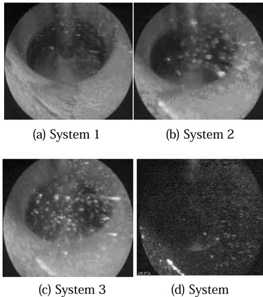
Figure 23 Droplet behavior with injection timing of IVO, IMEP; 400 kPa
